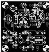
Figure 5. Printed circuit board for the lower frequency converter. The component side is a copper plane.
